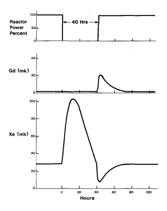
Figure 2: Gd Concentration in Moderator For a Start-Up 1-1/2 - 3 Days After a Shutdown
